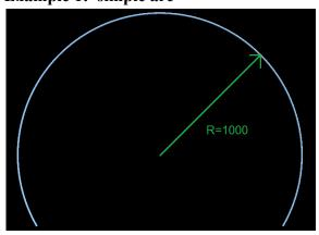
An arc with an arc radius of 1,000 mm (core dimension) and an angle of 240° will be represented via two segments:
