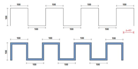
(The BF3D format is shown on top, the real iron geometry is shown below, when assuming that outer dimensions are specified in BF3D.)
