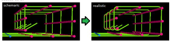
For bending angles of up to 90°, the bending shape simply is rather more "angular" than in reality. For bending angles above 90°, however, the outer shape will be shown distorted.
