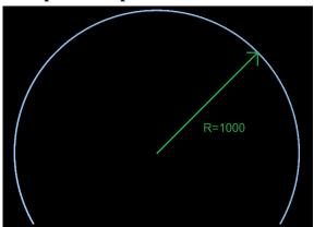
An arc with an arc radius of 1,000 mm (core dimension) and an angle of  $120^{\circ}$  will be represented via two segments:
