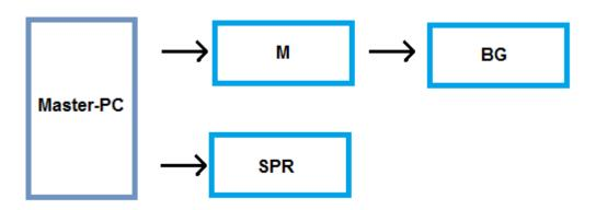
The machine M and the machine BG are cascaded, in the sense that BG is supplied by M with data. The control system ("Master PC") sends data in parallel to M and SPR.
