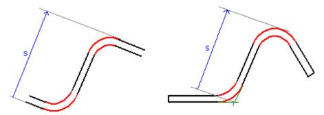
The **external length** of a segment is the segment's *external dimension* that runs in the direction of the segment. (The segment's external dimension is defined according to Section 1.6.16.4.).
