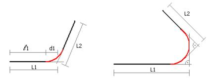
For angles not larger than  $90^{\circ}$ , R will have *no* effect on the bending shape, but merely results in the corners being rounded. The basic shape will then be given by the theoretical lengths. For bending angles beyond  $90^{\circ}$ , R will have a direct effect on the overall dimensions.
